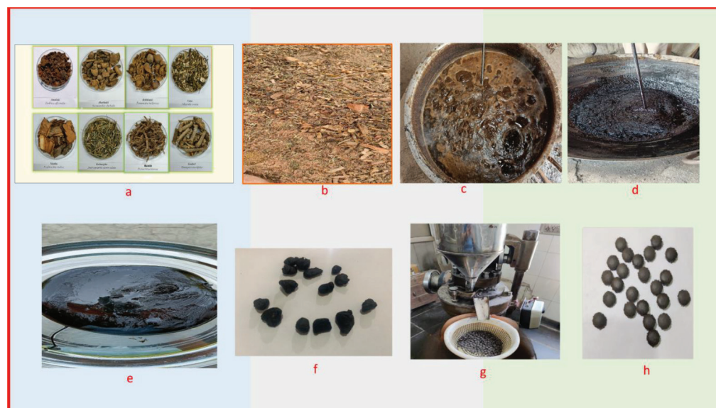
Figure 2. Sequential representation of the unit process of pharmaceutical preparation of Phalatrikadi Ghana vati ; (a) . Ingredients of PGV, (b) . Coarse powder of ingredients, (c) . Coarse powder is boiled with eight times of potable water till one-fourth of volume reduction to form decoction, (d) . Decoction is filtered and further reduced to a semi-solid consistency known as ghana , (e) . and (f) . Ghana is further dried to form granules for tablet compression, (g) . Tablet compression, (h) . Final product.
