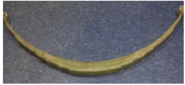
Figure 5. Mono-composite leaf spring.
