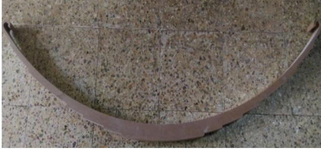
Figure 2. Pattern of mono-composite leaf spring.
