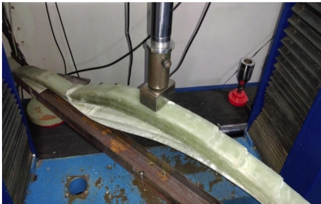
Figure 7. Failure of mono-composite leaf spring.
