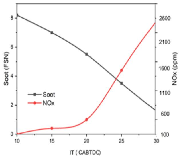
**Figure 12.** At 50.5% hydrogen and 0% EGR, the effect of injection timing on NOx and soot emissions was studied.
