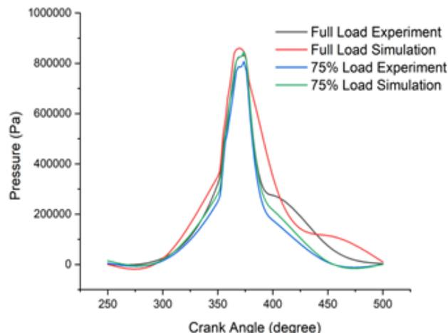
**Figure 2.** Pressure curve for the 7.45 l/min hydrogen/diesel mixture at 74% and full load.
