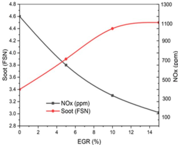
**Figure 9.** Soot and NOx emissions vary with EGR level of 50.5%hydrogen and 10 CA BTDC injection timing.
