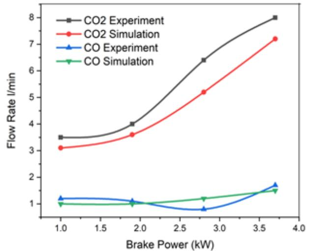
**Figure 5.** Variation in CO and CO<sub>2</sub> emissions for a 20 l/min H<sub>2</sub> flow rate with brake power.
