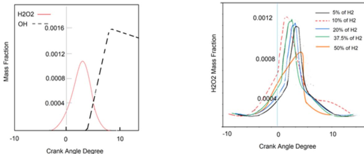
**Figure 8.** Variation in species mass fraction as a function of crank angle.
