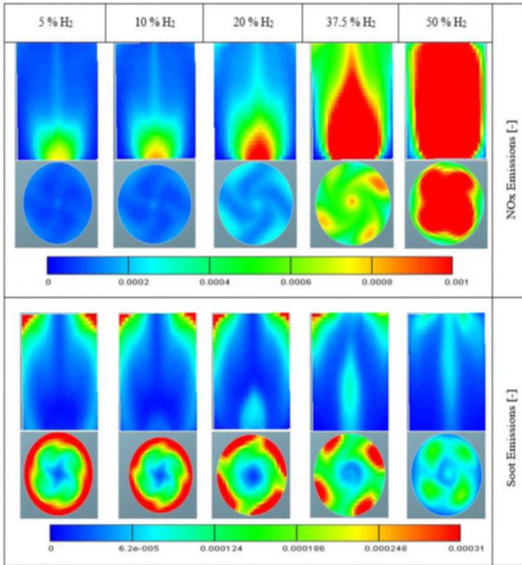
**Figure 7.** Effect of hydrogen concentration on soot and NOx emissions inside the engine cylinder at 0% EGR and 10 CA BTDC injection timing.
