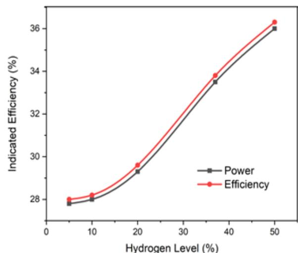
**Figure 6.** Engine power and efficiency with 0% EGR and 10 CABTDC injection timing as a function of hydrogen level.
