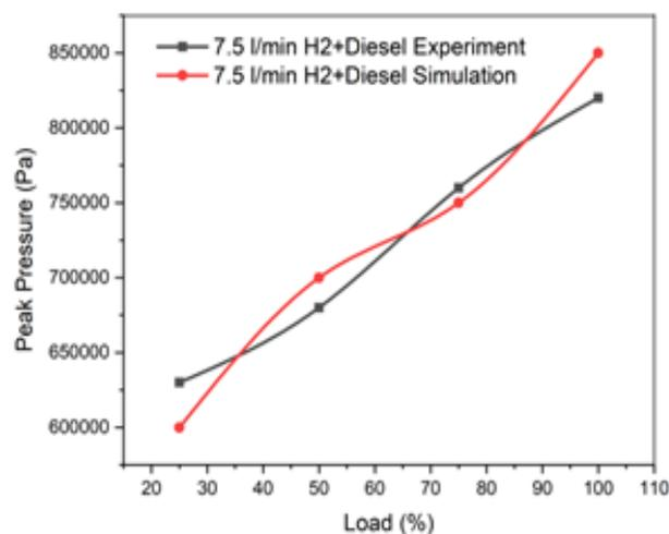
**Figure 3.** Peak pressure variation with loads at 7.45 l/min H<sub>2</sub> flow rate.
