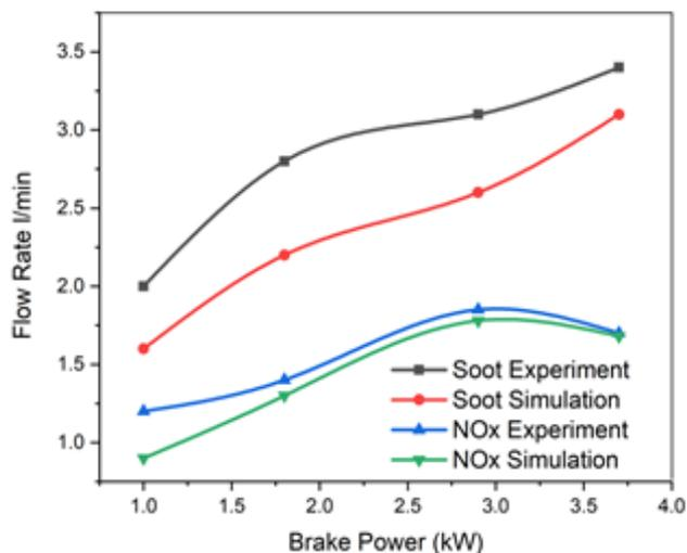
**Figure 4.** Soot and NOx emissions fluctuation at a 20.5 l/min H<sub>2</sub> flow rate with brake power.
