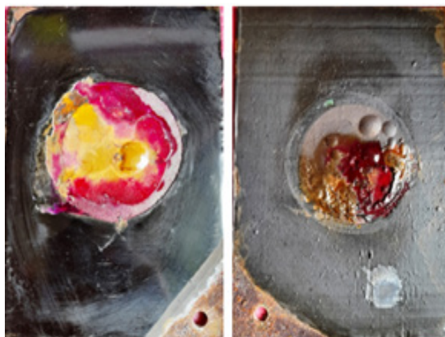
Figure 7. Images of MS coated panels after cathodic disbond test for 28 days.
