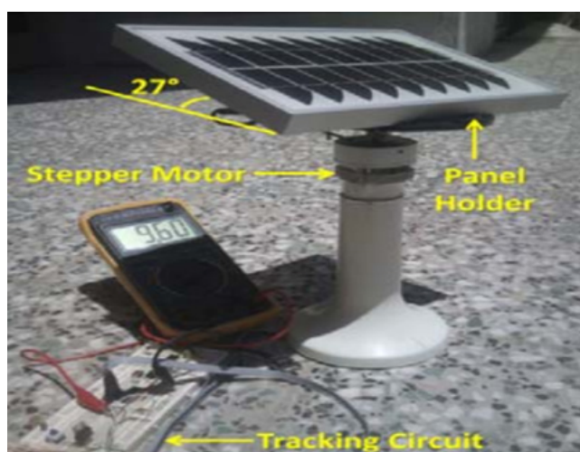
Figure 7. TSAT setup designed by Rezaei et al. , 13 .
