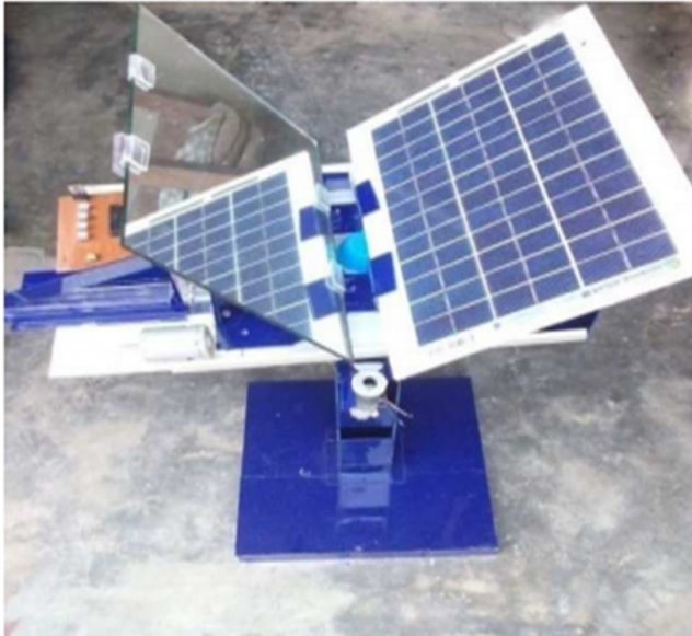
Figure 3. Mounting a mirror on a solar panel system 5 .
