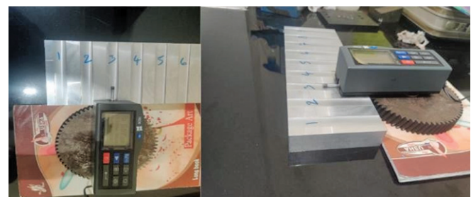
Figure 7: Surface roughness determined with the help of TIME3200 surface roughness tester (TR200)
