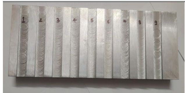
Figure 4: Nine slots milled at the top surface of Al-Li work piece
