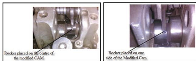
Figure 9: Rocker placed at different locations of tri lobed cam
