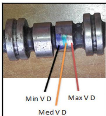
Figure 8 Magnified view of various displacement positions
