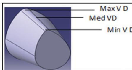
Figure 2: Valve displacement positions on cam profile
