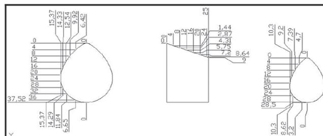
Figure 3: Angular positions of cam profile
