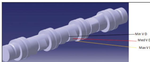
Figure 5: Modified cam shaft showing minimum, medium and maximum valve displacement positions
