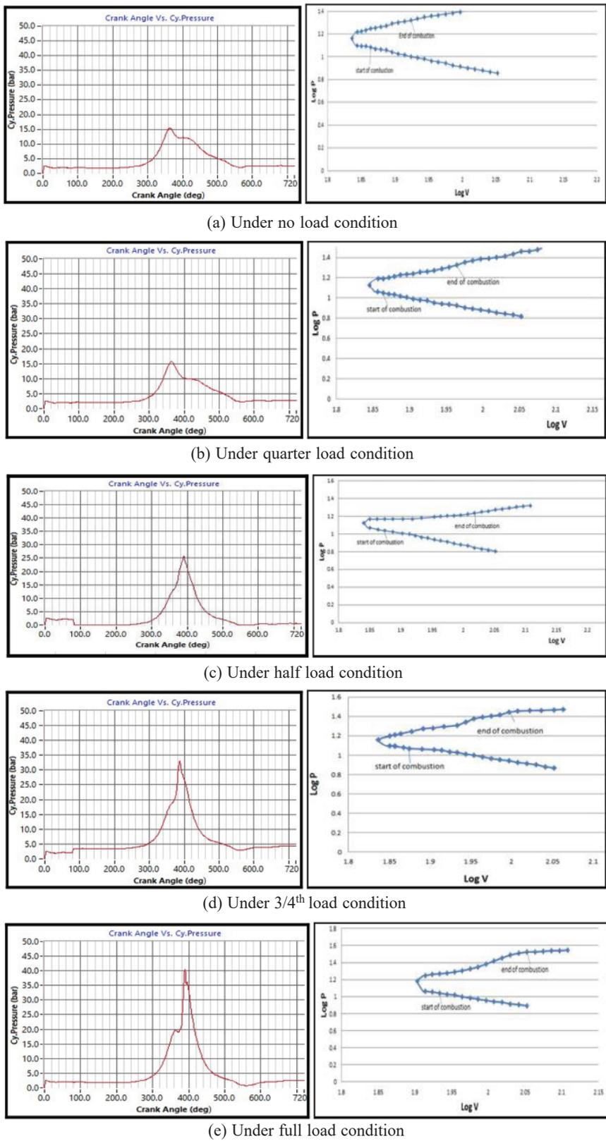
Figure 10: Pressure-Crank angle and Log P-Log V for 8° Taper turn in cam for different loading conditions
