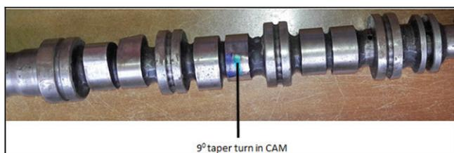
Figure 7: Modified shaft with 9° Taper turn in cam shaft
