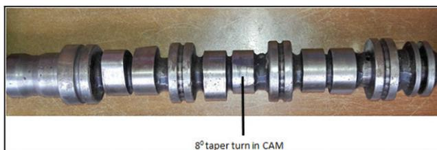
Figure 6: Modified shaft with 8° Taper turn in cam shaft
