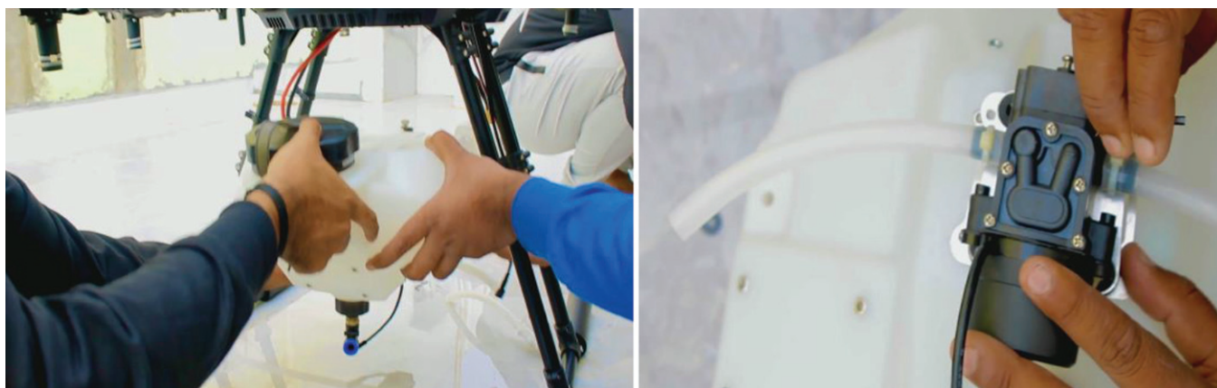
Figure 4: Hexacopter attached with tank and pump
