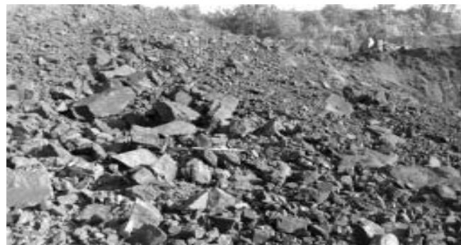
Fig.5 View of blasted muck pile due to blast conducted at 576 RL bench of Hill No.5
