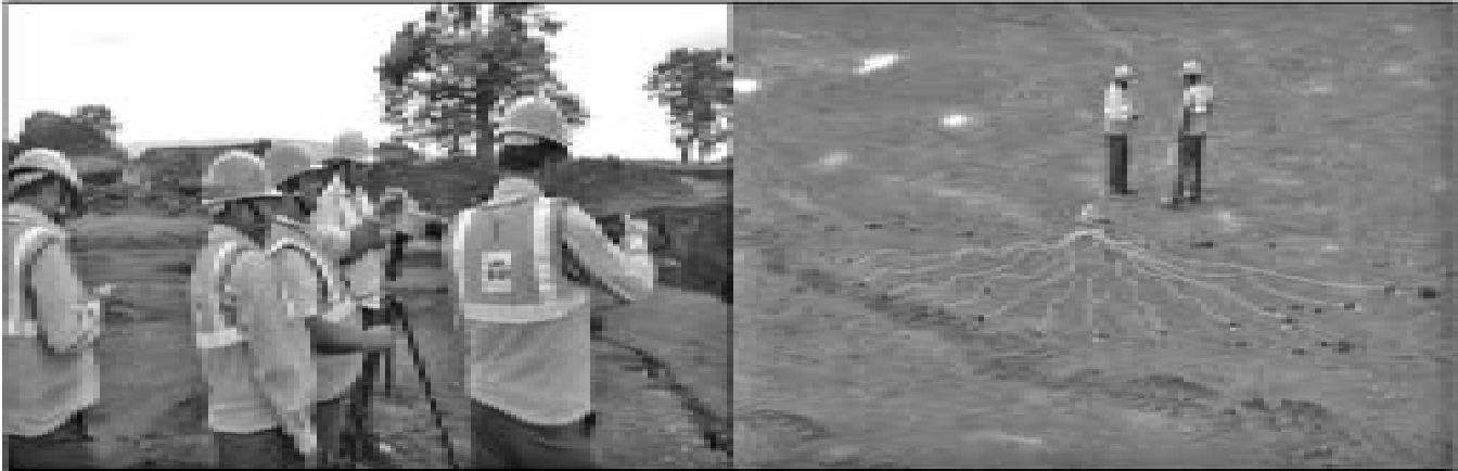
Fig.1 View of Nonel delay detonators connection arrangements for delay scattering test with the help of high speed camera
