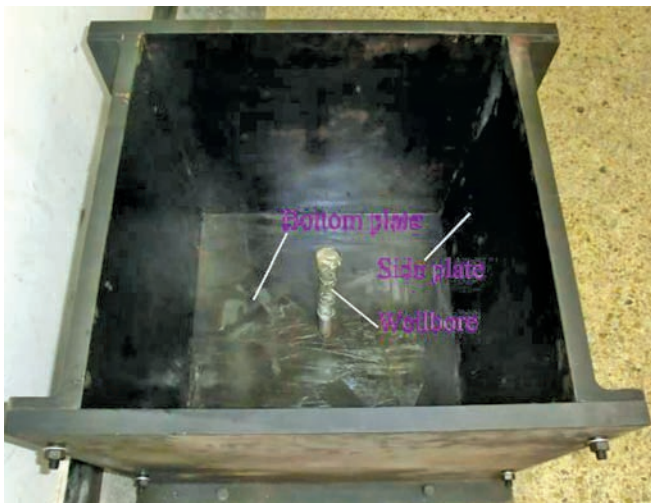
Fig.3 Rock sample mold and simulated wellbore
