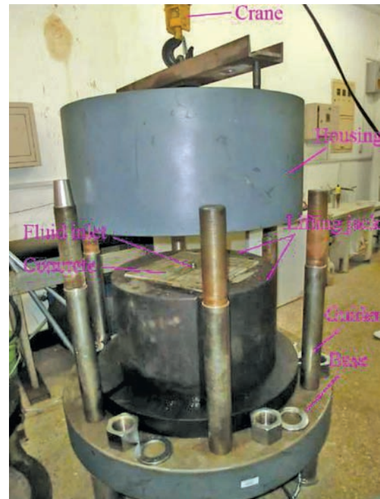
Fig.1 400 mm 3 true tri-axial hydraulic fracturing test equipment
