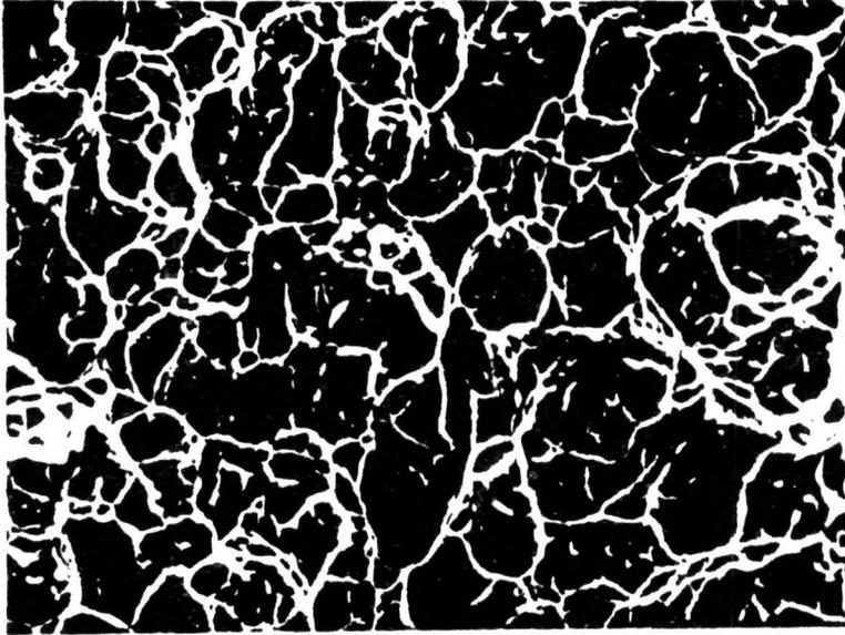
Fig. 6 : Base metal fractograph (SEM), 500X
