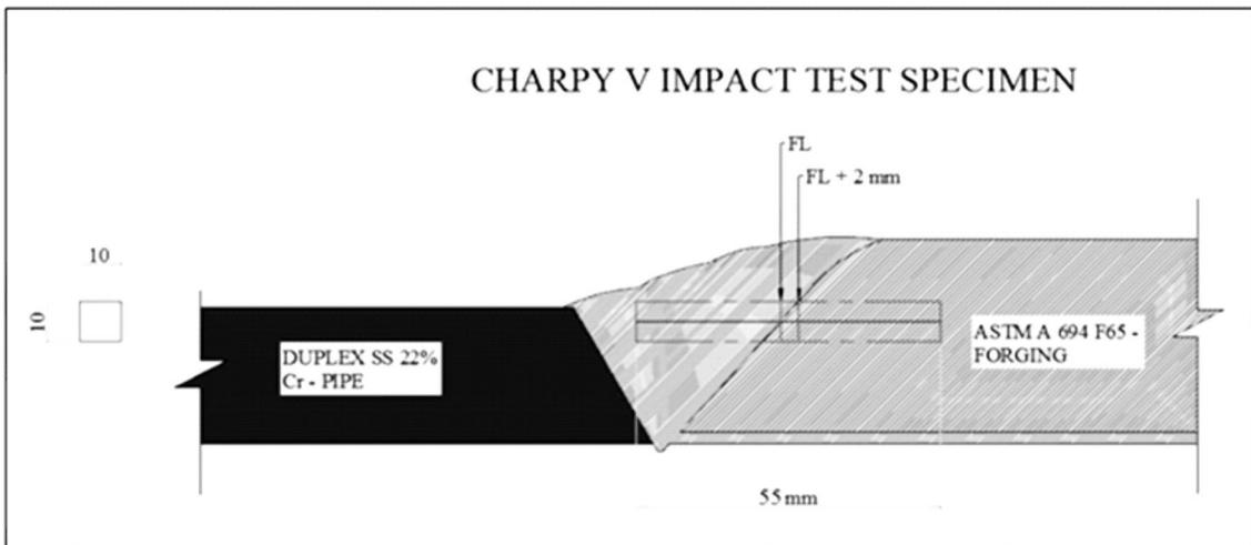
Fig 3.3 : Charpy-V Specimen at forging side fusion line +2mm
