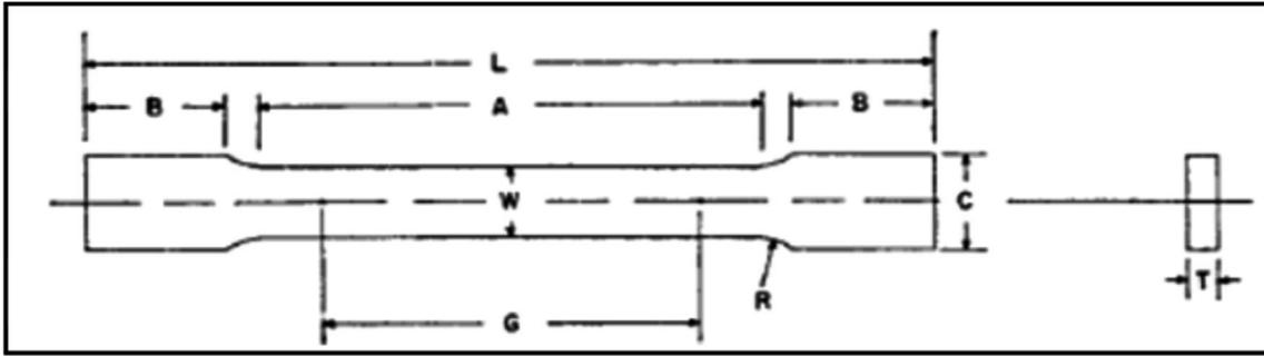
Fig. 2.1 : Rectangular Tensile test specimen as per DNV-OS-F101: 2010, Appendix B, A-400
