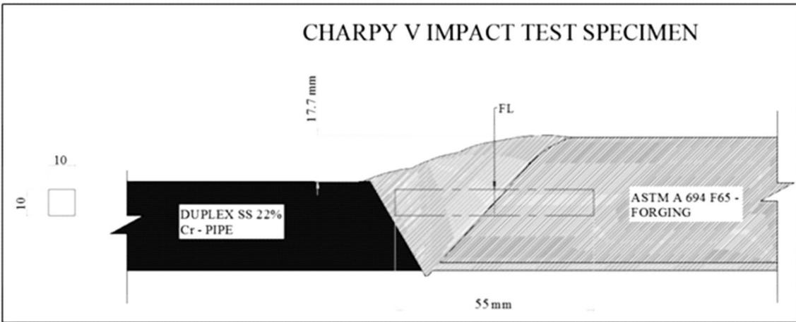
Fig 3.2 : Charpy-V Specimen at forging side fusion line
