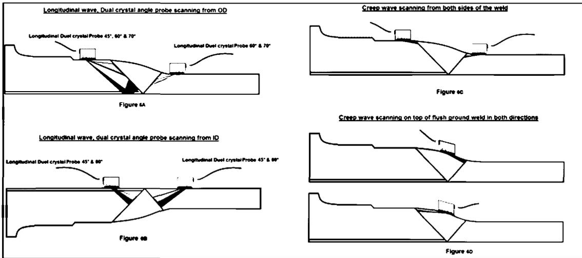
Fig. 6 : Final Scan plan established by using the mock-up & reference blocks (Figure 5& 2A to 2D)
