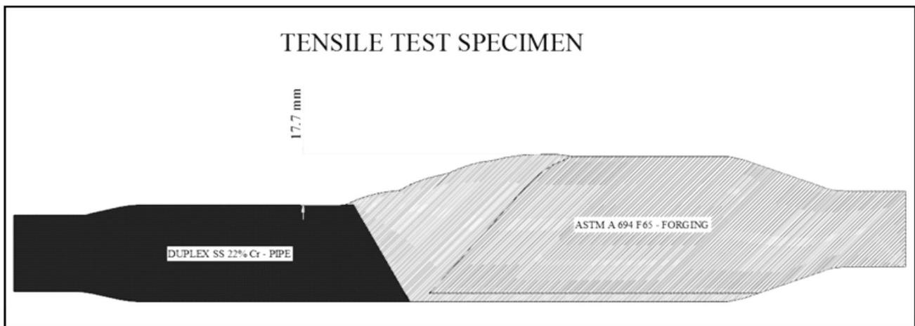
Fig.2.2 : As welded Tensile Test Specimen
