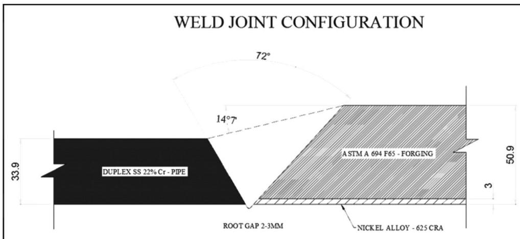
Fig.1 : Weld Joint Configuration
