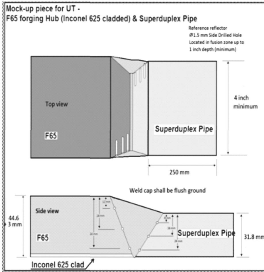
Fig. 4 : Mock-Up Test sample for UT
