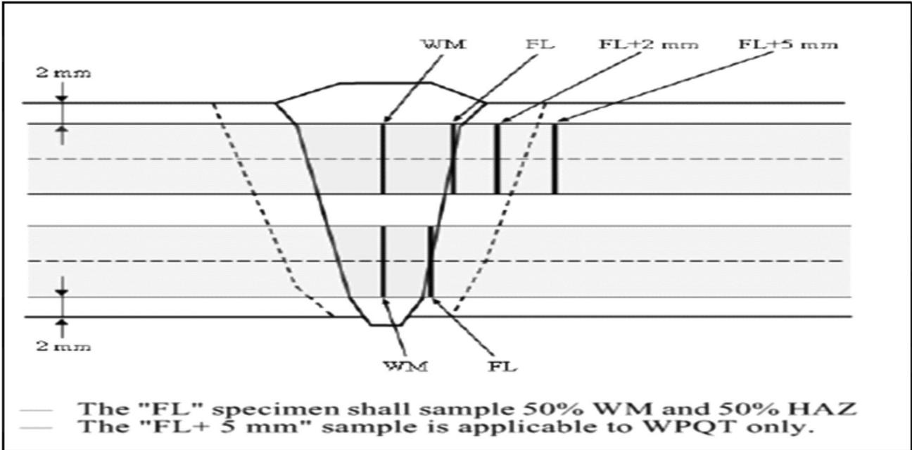
**Fig. 3 : Charpy V-notch impact test specimen positions for single sided welds with t > 25 mm as per DNV-OS-F101: 2010, Appendix B, A-500**
