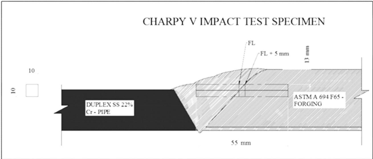
Fig 3.4 : Charpy-V Specimen at forging side fusion line +5mm
