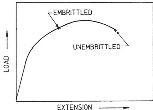
Fig. 1 . The effect of LME on the load Vs extension diagram (Schematic)
