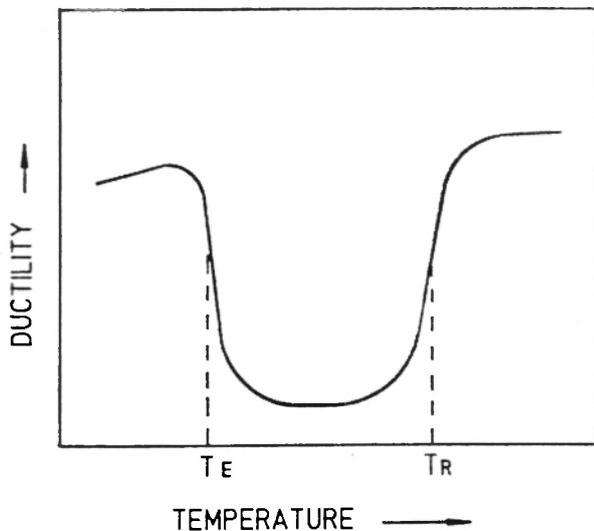
Fig. 2 : The effect of LME on the variation of Ductility with temperature (Schematic)
