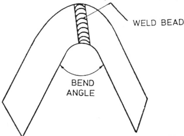
Fig. 9 . Schematic figure showing weld deposition of embrittler on the convex surface of a bent plate
