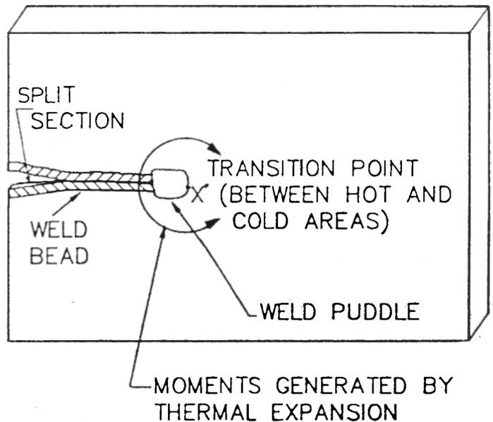
Fig. 3 : Weld Splitting Model
