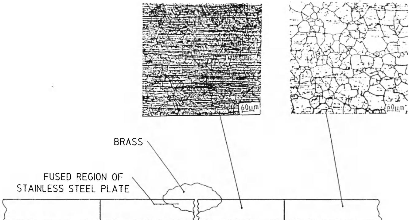
Fig. 18 Desensitisation effect produced in sensitized stainless steel plate as a result of welding
