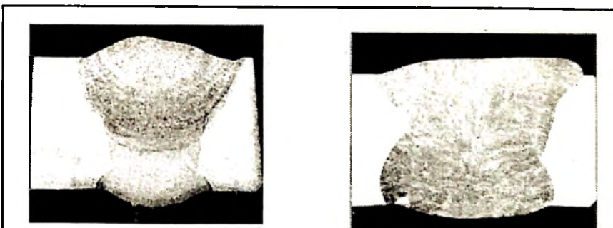
Fig. 3a Typical gas-shield flux-cored arc weld (GSFCAW) (4x)
