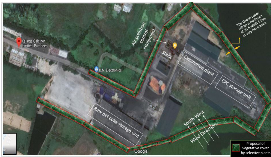
Figure 8. A 25 ft (8m) width green cover of large and long plants having 1 tree in every 6 m 2 is proposed to arrest the fugitive dust from the plant to spread out to the surrounding (please see the green belt around).
