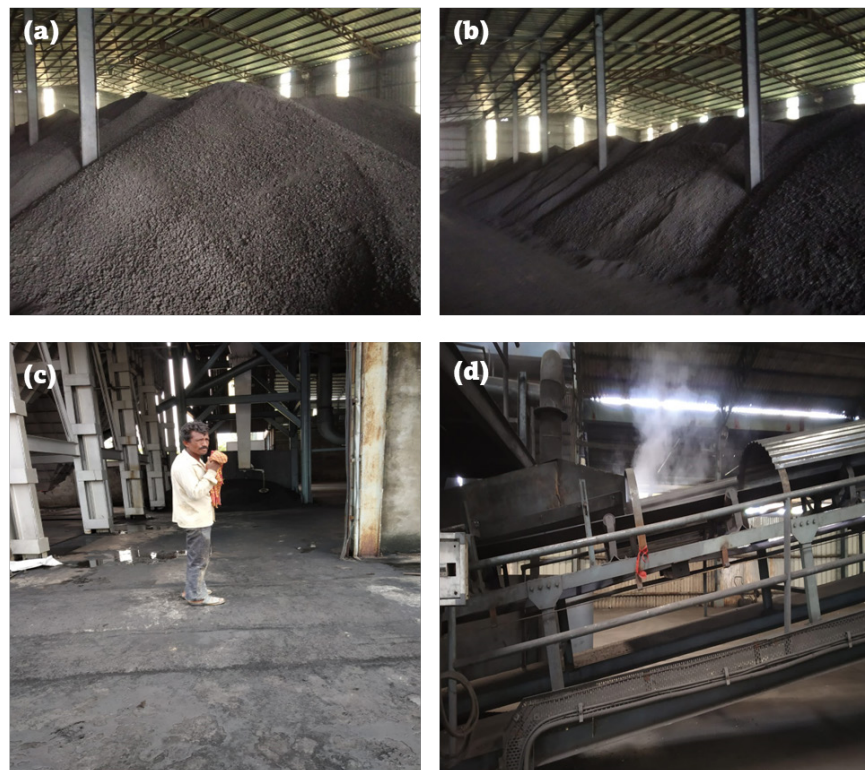
Figure 6. (a, b) Un-separated stockpiles contribute to fugitive dust exposure to the workers, (c) Worker without face mask, the image showing dust settled on the face, (d) Dust getting suspended in the air through open sections. The whole section can be flexibly covered.
