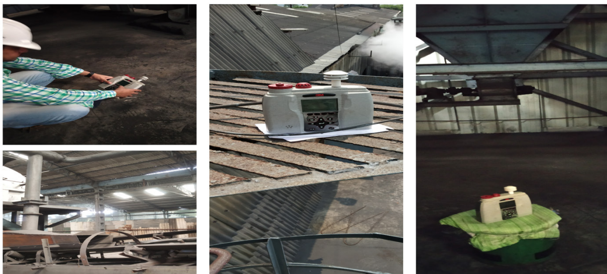
Figure 4. Indoor air pollution measurement by EVM 7.
