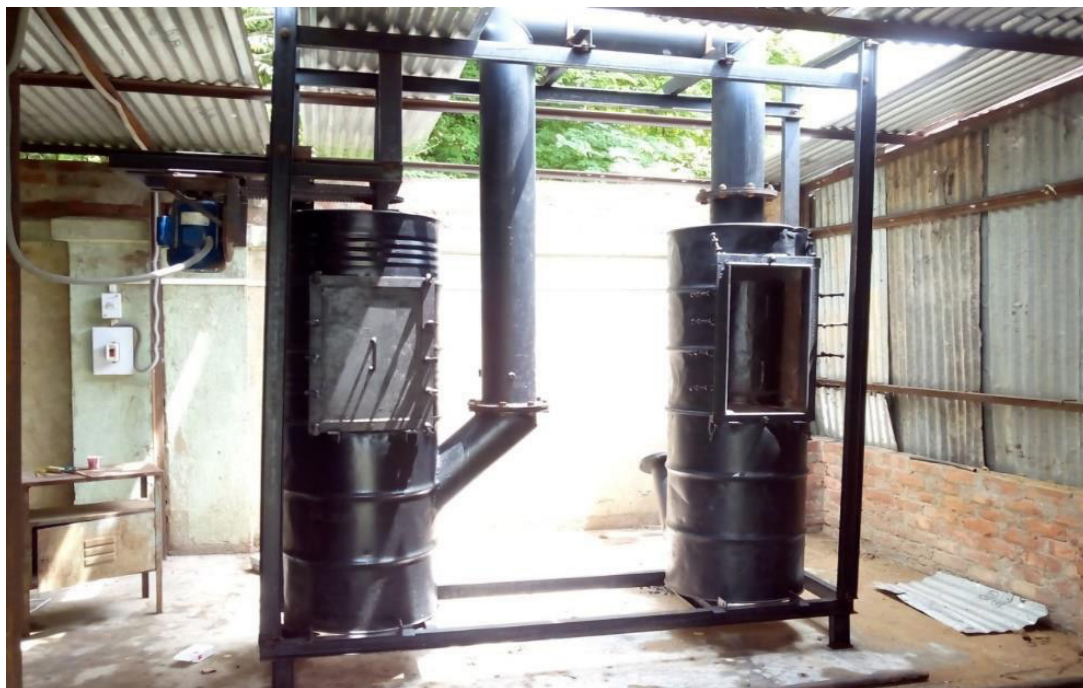
Figure 7. Slow pyrolysis setup for biochar production designed and fabricated at the School of Environmental Science and Engineering, Indian Institute of Technology Kharagpur. (Reproduced from Chandra et al. 26 with permission under the license agreement: 5861810142943)
