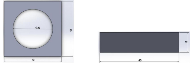
Figure 11. Top view and front view of upper and bottom components of mould.
